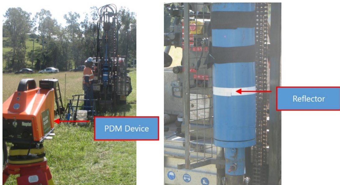
Figure 1. PDM obtaining data with reflectors on SPT hammer
